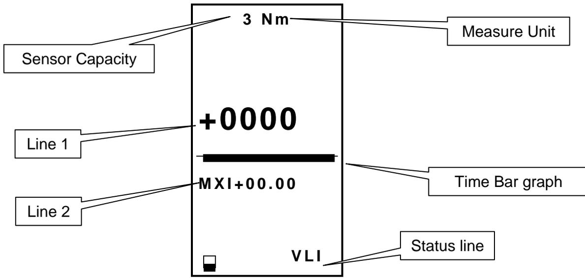
When turned on, CENTORMETER force gauge displays a small square in the middle of main screen (line 1). This small square slides from left to right and then the value of the force applied to the force gauge sensor appears on line 1 in big letters. If no force is applied, CENTORMETER force gauge displays « 0 ».
