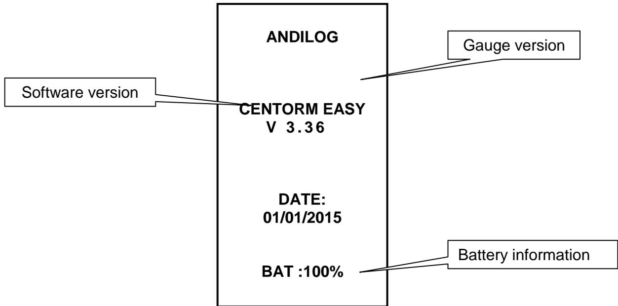
**Software version:** the line indicates the software version installed on the force gauge.
